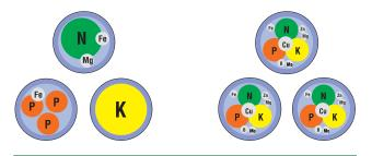
**Figure 4.** Comparison of conventional (only mixed) and EIRICH granulate. Left: conventional granulate with different composition of the granules. Right: EIRICH granulate (each granule contains the complete nutrient composition).
