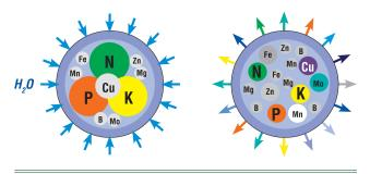
**Figure 5.** Nutrient release. Left: every fertilizer granule contains all the nutrients; the nutrients are dissolved by water. Right: a concentrated nutrient solution is created; the nutrients are released in a controlled manner.
