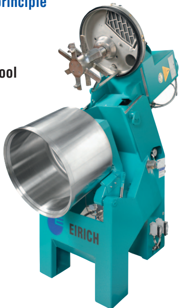
Laboratory mixer, 40 liters capacity
